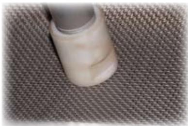
Opening the scanning nozzle to atmospheric pressure forces water from the clean side of the screen into the nozzle in a concentrated, high-speed stream, taking the filter cake with it.
