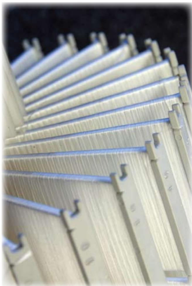
Concentrated streams of water automatically clean this thread filter, eliminating the need to replace cartridges or bags.
