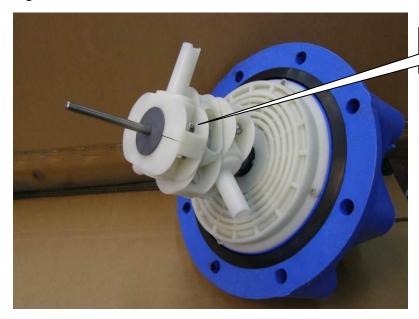
Remove bolts and nuts to replace nozzle
