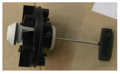
Valve and Turbine Assembly (shown with Allen wrench)
