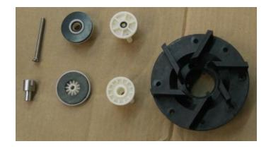
6. Take care that rubber seals and valve parts face the correct direction when assembling.
