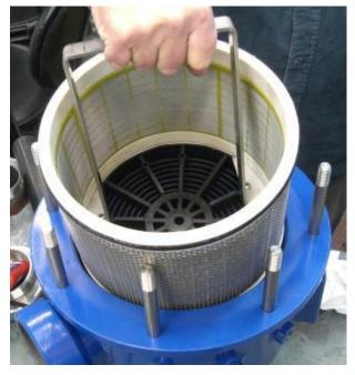
3. Using the special tool, pull the screen out of the housing. (CAT. NO. 710103-001121- TOOL EXTRACTOR M100 S/ST304 F/FINE SCREEN)
