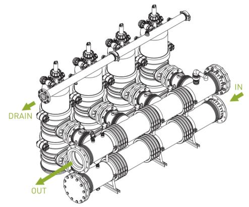
Sigma Pro 6" installation of 2 units with manifold, for flow rates up to  $360 \text{ m}^3/\text{h}$  (1,584 gpm)
