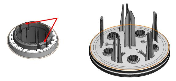
3. To assemble, attach the new bushing to the Sigma Pro multi-tool and insert into top plate. Rotate and click to lock.
