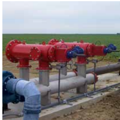
District water, 1,800 gpm, 100 micron, protecting drip tape irrigation
